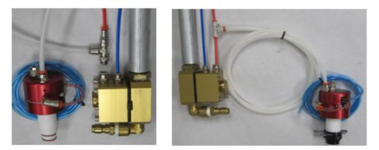
PPVS Valve to MPG connection for 4mm MPG tube – replace existing fitting with Tee and Reducer then connect to PPVS leak port. The port can be blocked when the PPVS is not in use. Another option is shown using the 4mm Tee to connect to PPVS leak port.
