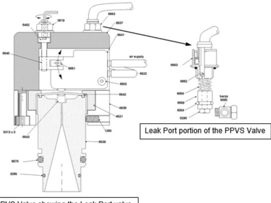
PPVS Valve showing the Leak Port valve
