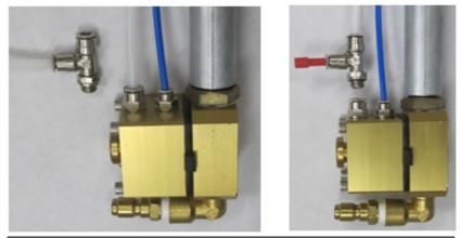
PPVS Valve to MPG connection for 6mm MPG tube – replace existing fitting with 6mm Tee and connect to PPVS leak port. The port can be blocked when the PPVS is not in use.
