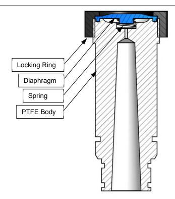
Once the PPVS is completely reassembled, test its function. If no test device is available, connect the air supply and the output to the TAS and suck the clean end of the PPVS to test if it functions correctly.
