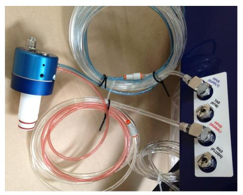
Figure 2. PPVS-INF to Innovator II Control Box
