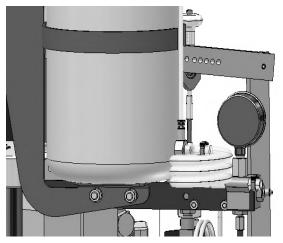
Figure 1. Catalyst Jug Bracket & Manifold
