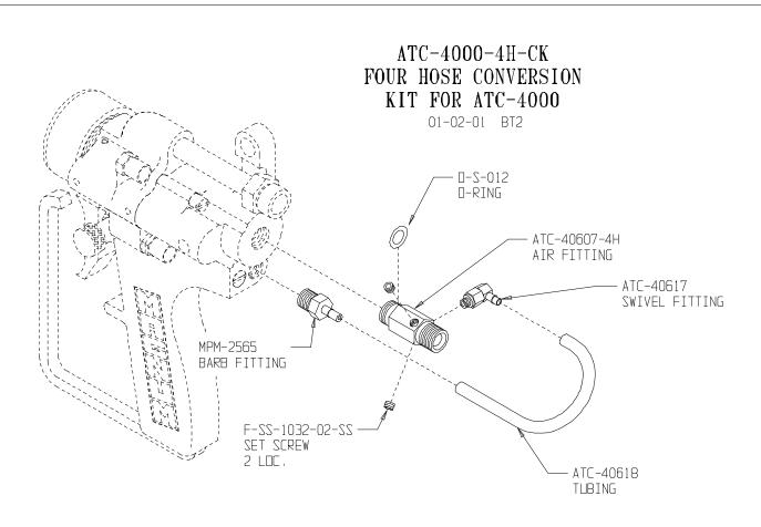
NOTE: INSTALL ATC-40607-4H TO DETERMINE WHERE THE OPEN TAPPED HOLES WILL BE. INSTALL THE ATC-40608 IN AN OPEN HOLE ON THE RIGHT SIDE. ITS POSITION WILL VARY. PLUG THE OTHER HOLES WITH THE SET SCREWS AND LOCTITE. DO NOT USE TUBING TO HANG GUN.
