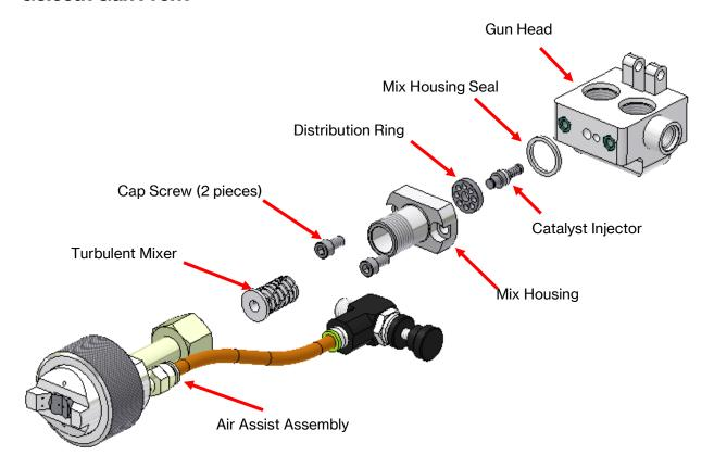
Note The TLN2-IG-200 gun uses the VPA-1000-VFIT air assist assembly and VFIT-XXXX spray tips. The TLN2-IG-100 gun uses the VPA-1000 air assist and ATG-XXX spray tips.
