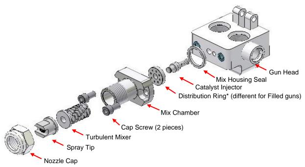
Note The TLN2-IC-100 and TLN2-IW-100 guns use the FT-XXX or N-XXXXC airless spray tips.
