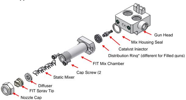
Note The TLN2-IC-200 and TLN2-IW-200 guns use the VFIT-XXXX FIT spray tips.
