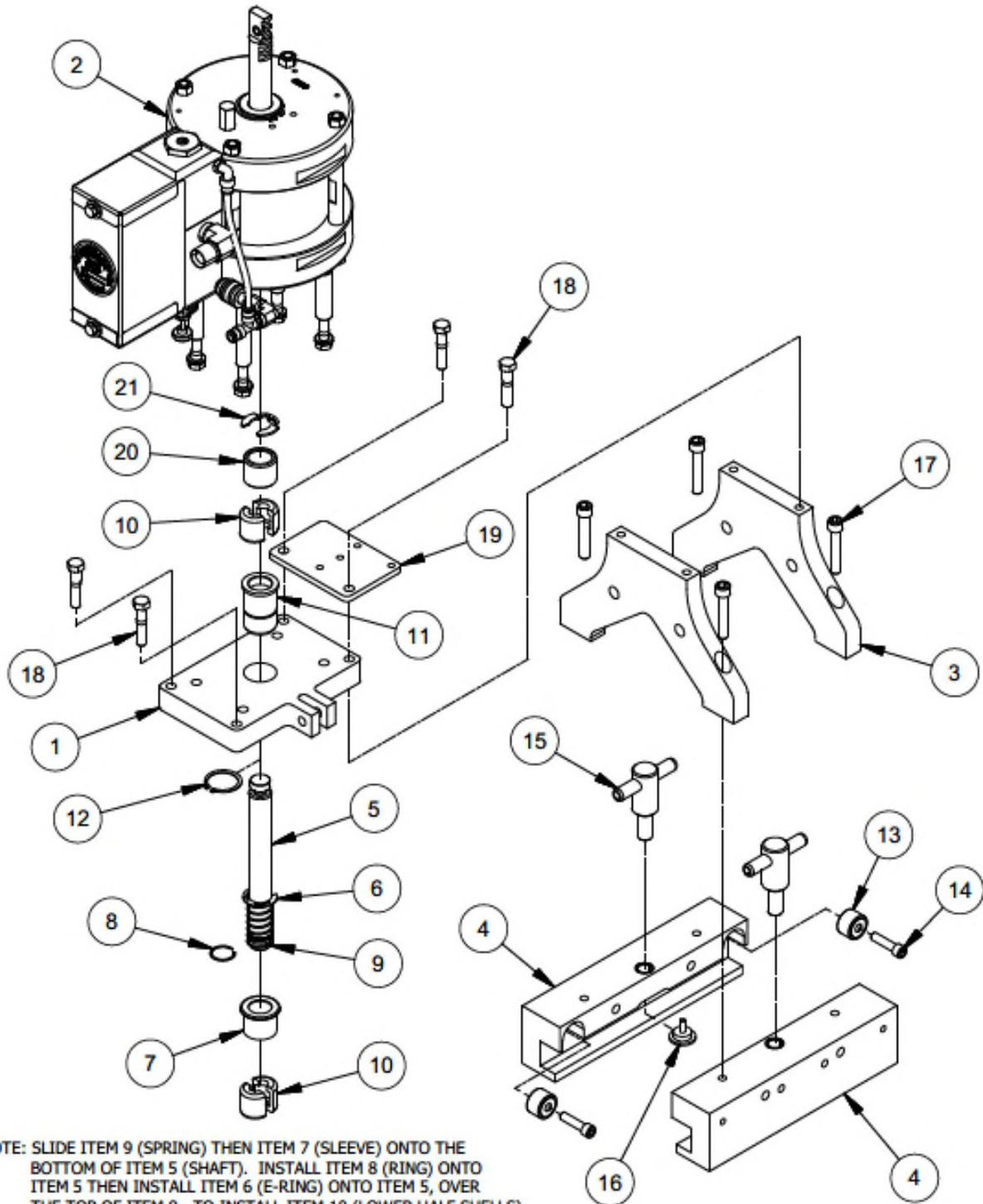
NOTE: SLIDE ITEM 9 (SPRING) THEN ITEM 7 (SLEEVE) ONTO THE BOTTOM OF ITEM 5 (SHAFT). INSTALL ITEM 8 (RING) ONTO ITEM 5 THEN INSTALL ITEM 6 (E-RING) ONTO ITEM 5, OVER THE TOP OF ITEM 9. TO INSTALL ITEM 10 (LOWER HALF SHELLS), SLIDE ITEM 7 UP TO COMPRESS SPRING.
