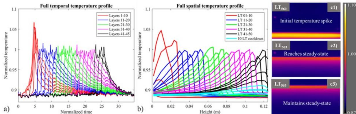
Figure 6. a) Normalized temperature vs. time for LT<sub>563</sub> (every other layer). b) Normalized temperature vs. height for LT<sub>563</sub> (every two layer intervals). c) IR thermal evolution for LT<sub>563</sub>.
