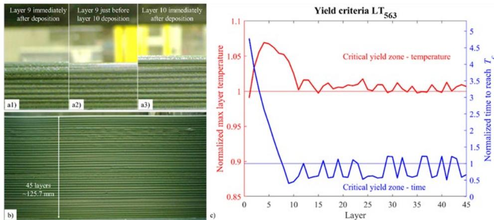
Figure 7. a) Yielding behavior of layer 9 due to the initial temperature spike, followed by deposition of layer 10. b) Full successfully printed wall. c) Normalized max temperature and time to  $T_c$  vs. layer to identify yield criteria.
