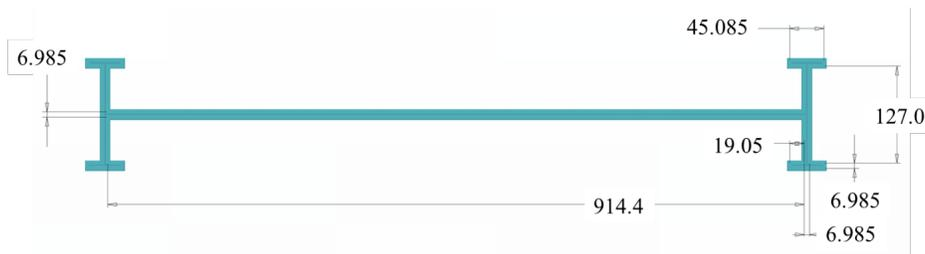
Figure 2. Semi-infinite, thin-wall specimen schematic with dimensions (mm).
