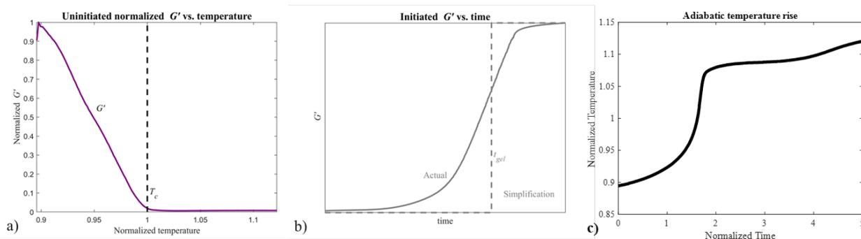
Figure 5. a) Storage modulus of Polynt thermosetting resin as a function of temperature b) Conceptual plot of “actual” and “simplified” behavior of  $G'$  with time c) Adiabatic temperature rise data from experiment showing exothermic behavior.
