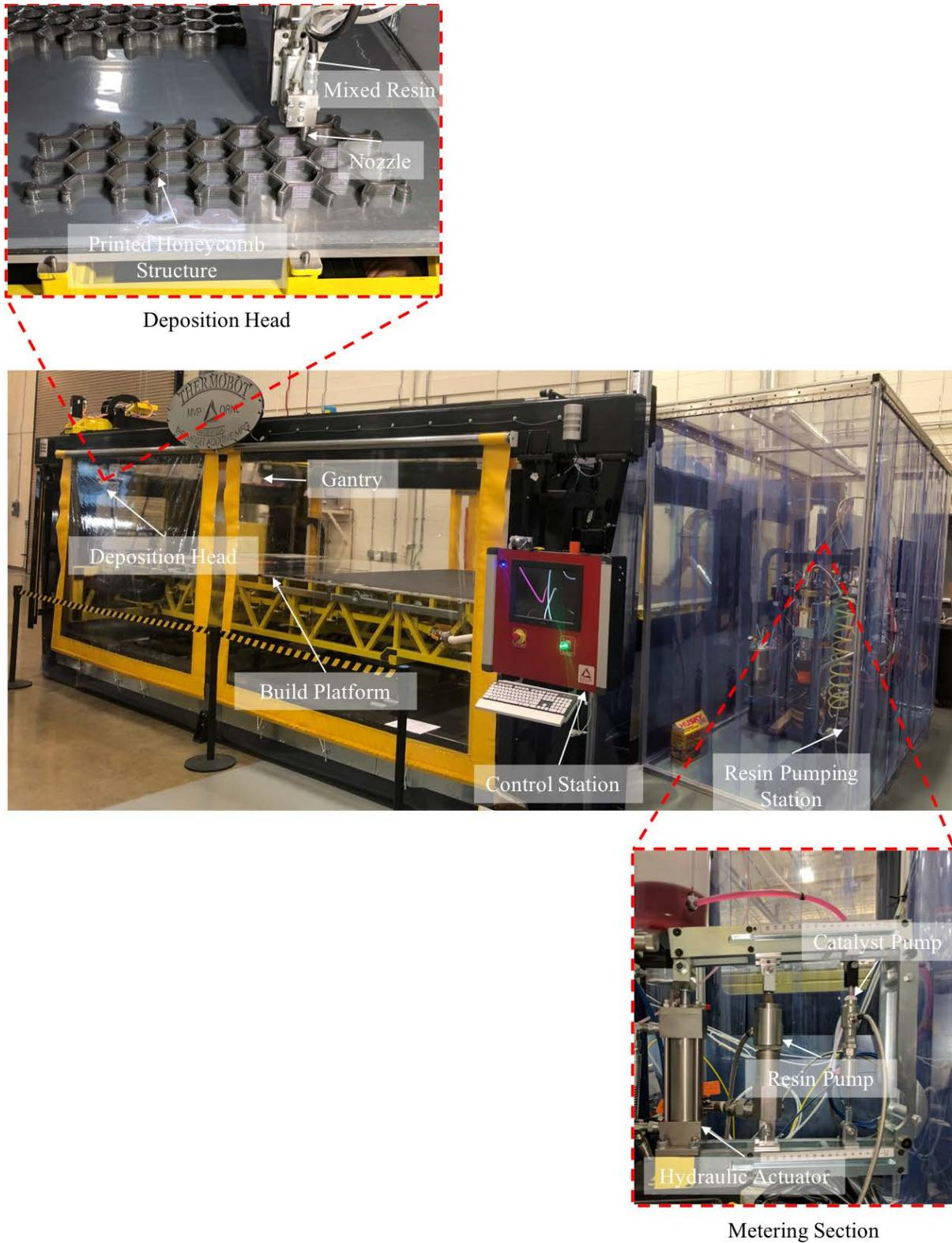
Figure 1: Large scale reactive polymer additive system showing the build platform, resin pumping station, and deposition head system
