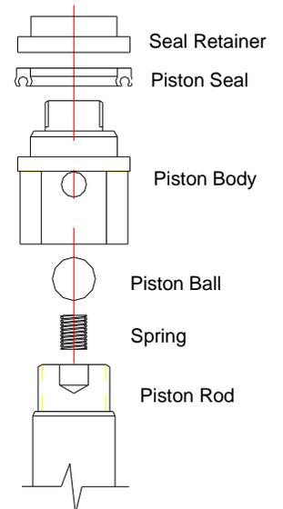
6. Slide the Piston Seal (VHPC-1222) onto the piston body with the cup side facing down. Screw the Seal Retainer (VHPC-1212) onto the piston body. Remove from the vise and set aside for now.
