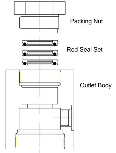
4. Take the assembled Outlet Body and with a twisting motion push it onto the Piston Rod. The Packing Nut (VHPC-1207) should go on first so that it is pointing down. A little force may be required to go through the seals.
