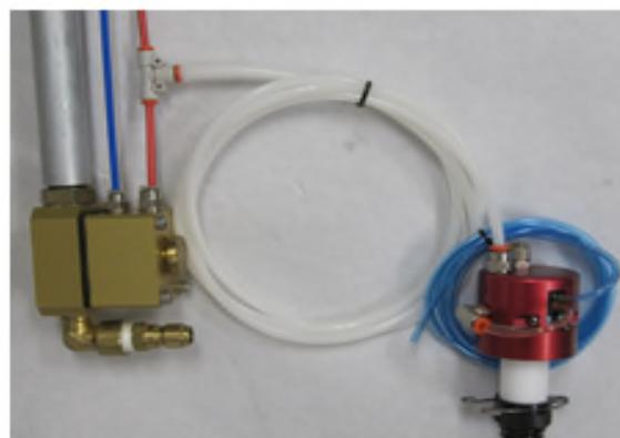
PPVS Valve to MPG connection for 4mm MPG tube – replace existing fitting with Tee and Reducer then connect to PPVS leak port. The port can be blocked when the PPVS is not in use. Another option is shown using the 4mm Tee to connect to PPVS leak port.
