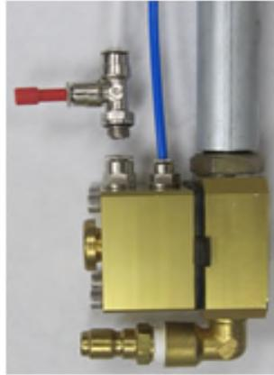
PPVS Valve to MPG connection for 6mm MPG tube – replace existing fitting with 6mm Tee and connect to PPVS leak port. The port can be blocked when the PPVS is not in use.
