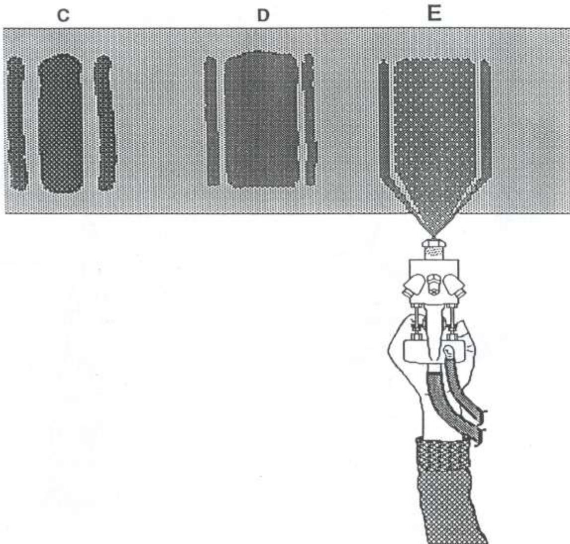
**D. The pattern is at or near full width:** There are well-defined fingers; however there is little or no white frothing (air bubbles) in the center of the sprayed material. Result "D" is a usable pattern for an experienced operator.
