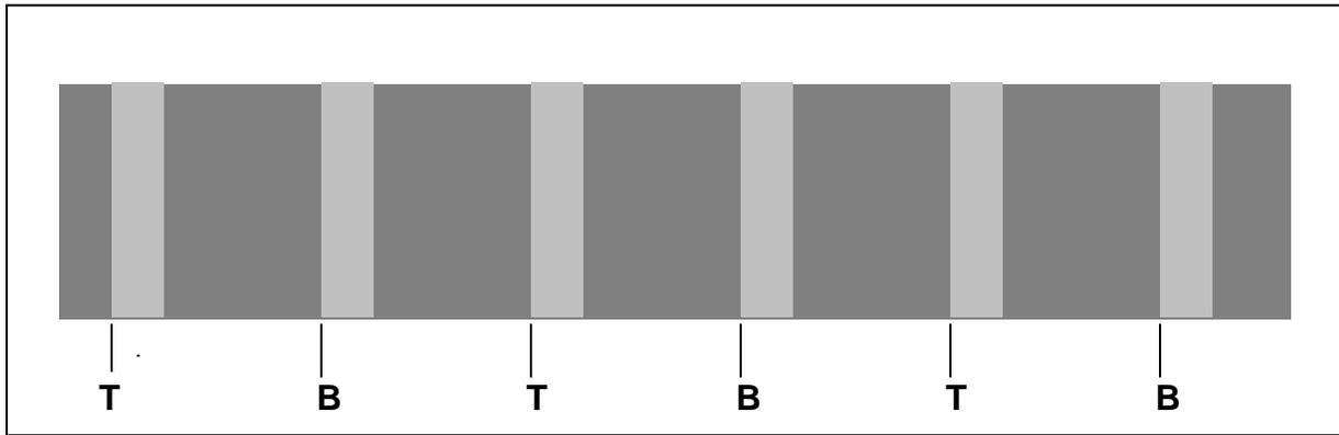
Improper cure at the top and bottom of the stroke indicates an accumulator issue either catalyst or resin.
