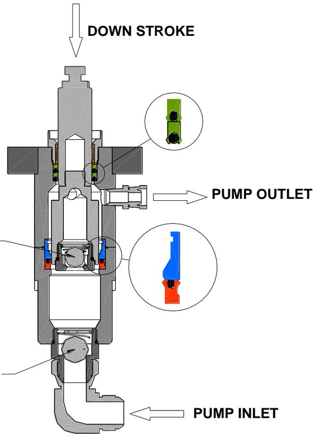
**UP STROKE:** The piston seal seals on the piston, the piston body ball seals in its seat; everything above the piston body is pushed out. A vacuum is created below the piston body and new material is drawn in.
