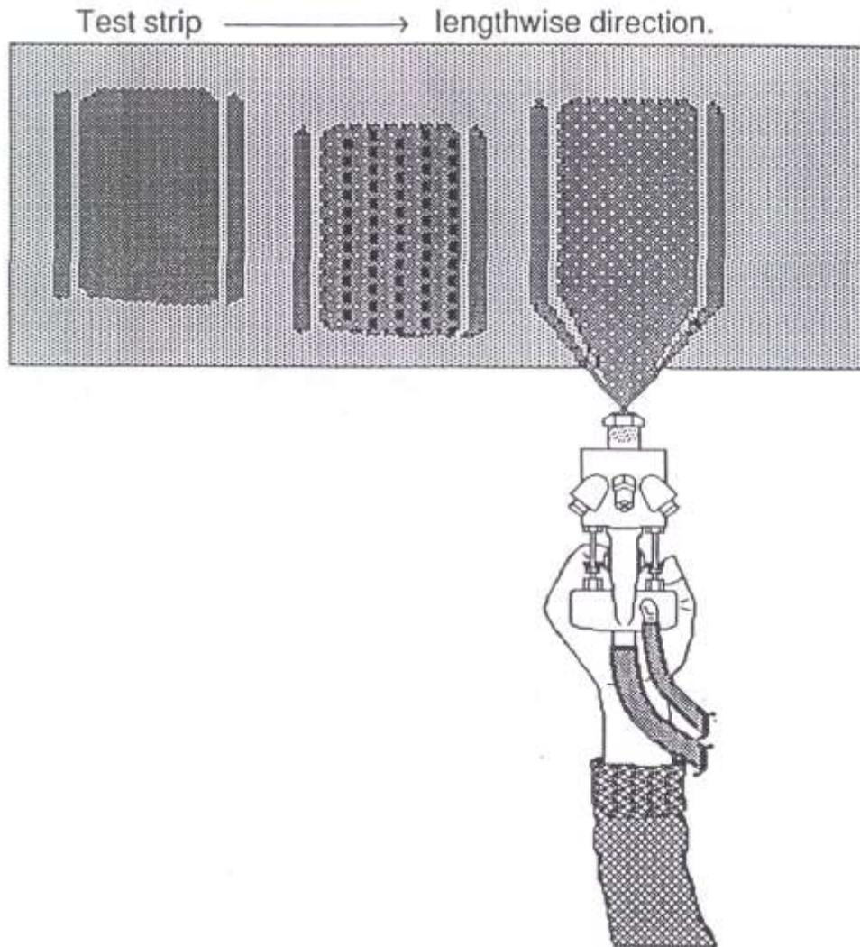
4. Flush the gun into an appropriate container after every test shot.
