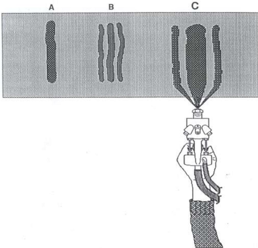
**B. Three heavy fingers:** Horns are beginning to develop, but the operating pressure is still very low.
