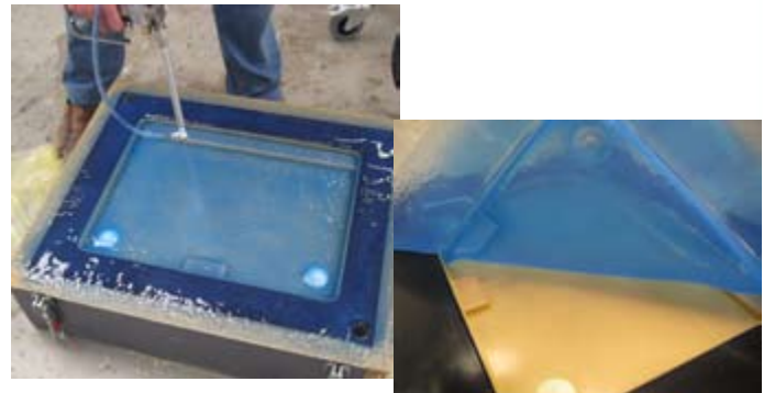
Producing the vacuum bag by spray method
